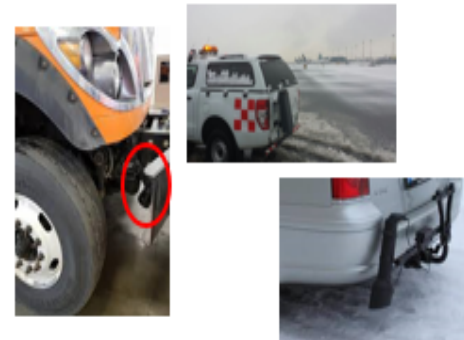
Mobile Sensor (provides all key parameters, including grip)
